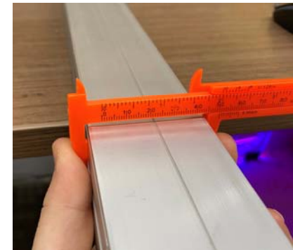
Figure 3: Photo here with caliper shown at an angle makes it unclear to determine caliper reading.
