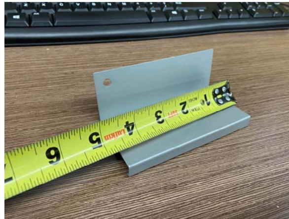
Figure 6: Photo here with tape measure shown at an angle makes it unclear to determine tape measurement reading.
