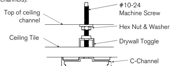
Place perforated steel angle over screws. Add final washer and nut, and hand tighten to secure. **Make sure ceiling tile does not deform when securing angle between nuts.**
