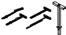
Using Phillips head bit, install #10-24 machine screws through C-bracket into toggles. If installing to a drop ceiling, continue to Step 6. Otherwise, proceed to Step 7.
